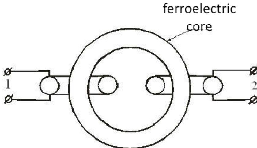
Figure 4: Transformer with the toroidal ferroelectric core
