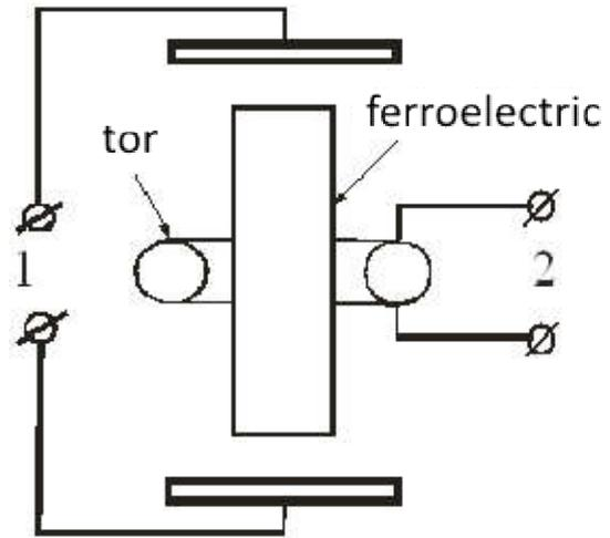
Figure 3: Schematic of ferroelectric transformer
