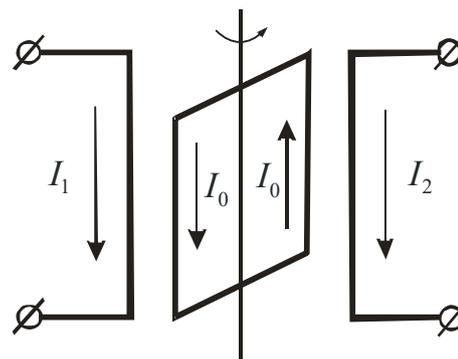
Figure 2: Transfer of the currents of induction of one conductor in another with the presence between them of ferromagnetic material
