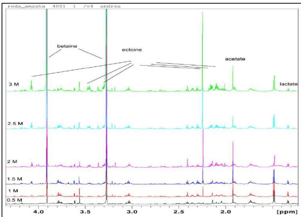
Figure 1: NMR <sup>1</sup>H spectra of cell extracts from *Halomonas aquamarina* at 0.5, 1.0, 1.5, 2.0 and 3.0 Na Cl (M) in saline nutrient medium spectra (Source Red Sea Sedimen)
