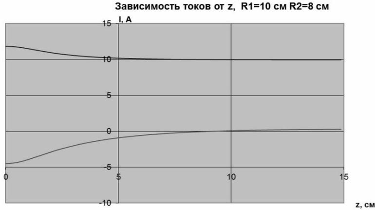
Fig. 1: Graphs of currents in the lower ring (upper curve) and in the upper ring (lower curve) with the initial values of current strength in the lower ring – 10 A and the value of current strength in the upper ring – 2 a.
