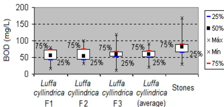
Figure 7: Box-whisker graphics for biochemical oxygen demand (BOD<sub>5,20</sub>) downstream the filters filled with *Luffa cyllindrica* (F1, F2, F3 and average value) and downstream the filter filled with stones (upstream the secondary settlers).
