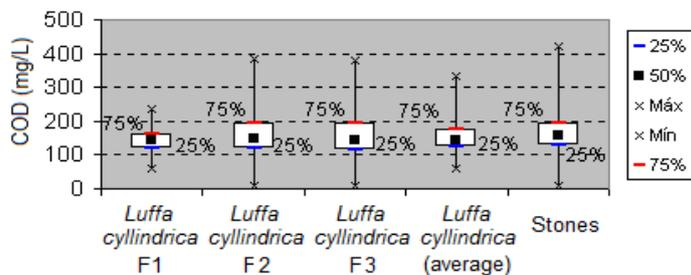
Figure 11 : Box-whisker graphics for chemical oxygen demand (COD) downstream the filters filled with *Luffa cyllindrica* (F1, F2, F3 and average value) and downstream the filter filled with stones (upstream the secondary settlers).
