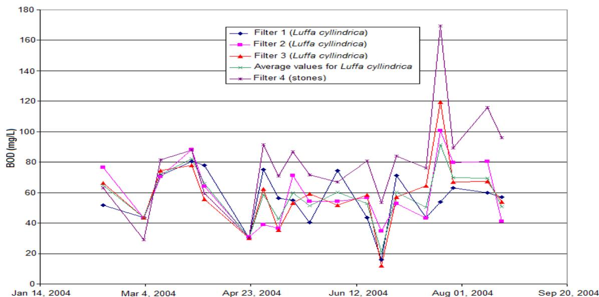
Figure 6 : Biochemical oxygen demand (BOD<sub>5, 20</sub>) downstream the trickling filters filled with *Luffa cyllindrica* (F1, F2, F3 and average value) and downstream the filter filled with stones (upstream the secondary settlers): temporal series.
