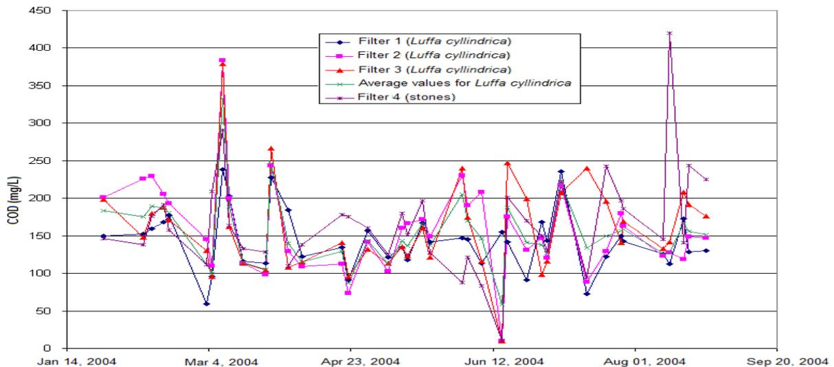
Figure 10 : Chemical oxygen demand (COD) downstream the trickling filters filled with *Luffa cylindrica* and downstream the filter filled with stones (downstream the secondary settlers): temporal series.
