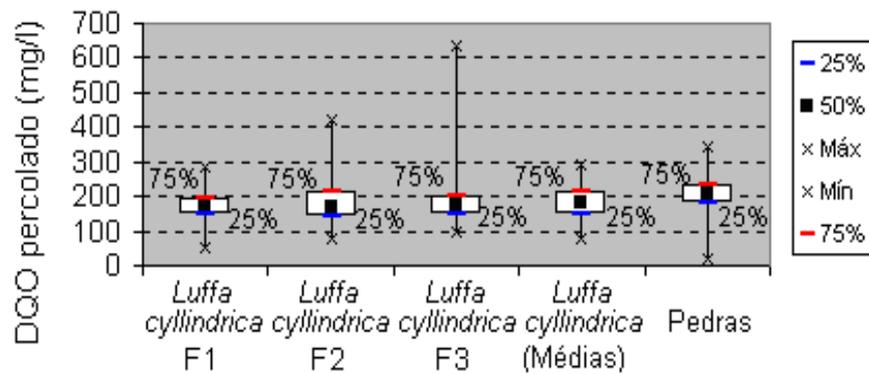
Figure 9 : Box-whisker graphics for chemical oxygen demand (COD) downstream the filters filled with *Luffa cylindrica* (F1, F2, F3 and average value) and downstream the filter filled with stones (upstream the secondary settlers).
