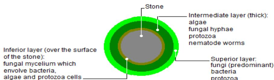
**Figure 3:** Composition of the biofilm on a trickling filter support medium, as described by Branco, 1976.
