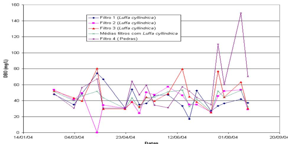
Figure 8: Biochemical oxygen demand (BOD<sub>5, 20</sub>) downstream the trickling filters filled with *Luffa cyllindrica* (F1, F2, F3 and average value) and downstream the filter filled with stones (downstream the secondary settlers): temporal series.
