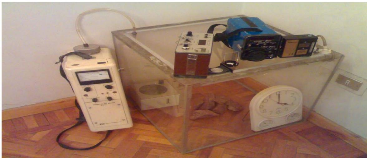
Figure 1 : Radon calibration chamber
